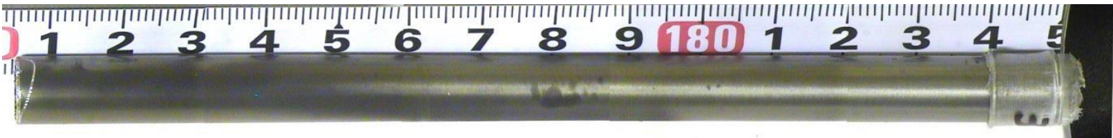
Visual inspection of CrN coated Zr-4 tube from IFA-774 – 180 degree
